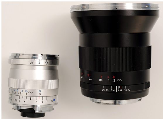
Size comparison of nearly symmetrical and retrofocus wide-angle lenses with the same focal length and maximum aperture.
