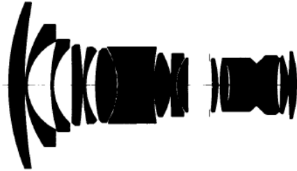
Lens cross-section of the Distagon 2.8/21 for the Contax SLR, a relatively complex lens with 15 elements in 13 groups. However, it had no aspherical surfaces. Its performance, particularly the perfect correction of lateral chromatic aberration, was achieved solely by the combination of very special (and expensive) high-index glass types with glass types displaying extremely high anomalous partial dispersion.
